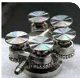
Rotation of individual target to prevent laser drilling
